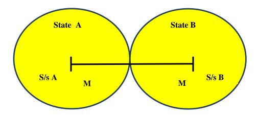
Net VArh exported from S/s-A, while voltage < 97% = X1Net VArh exported from S/s-A, while voltage > 103% = X2Net VArh imported at S/s-B, while voltage < 97% = X3Net VArh imported at S/s-B, while voltage > 103% = X4
